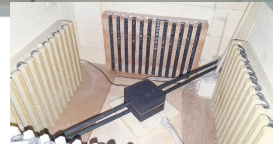
Sealed test-fixture for single cells
